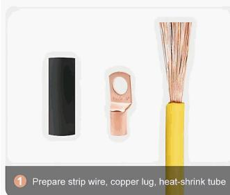
① Prepare strip wire, copper lug, heat-shrink tube
