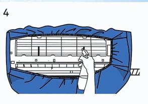
Connect the drain hose and start cleaning.
