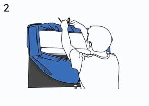
Unfold the elastic cord of the cleaning cover by hand and wrap it around the air conditioner.
