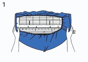
Hold the back of the support plate with your hand, prop open the cleaning cover, and slip it into the air conditioner.
