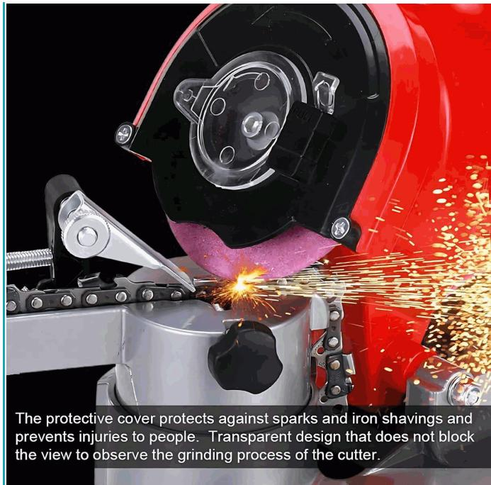
The protective cover protects against sparks and iron shavings and prevents injuries to people. Transparent design that does not block the view to observe the grinding process of the cutter.
