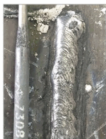
Z308 medium carbon steel, φ3.2 electrode
