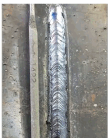
J422 mild steel φ3.2 electrode
