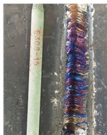
E308 Stainless steel φ3.2 electrode
