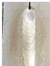
Joint 8mm steel plate with φ3.2 electrode
