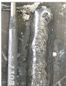
Z308 medium carbon steel, φ3.2 electrode
