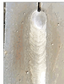
Joint 8mm steel plate with φ3.2 electrode
