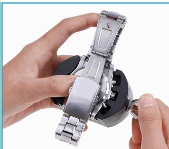
Adjust the fixator to fix watch
