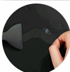
Exhaust the air with scraper
