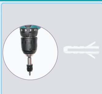
Step 2: If using a plastic wall anchor, pre-drill a 0.2in hole and tap. Place assembly into position and install screw in anchor; if using screw only, pre-drill a 0.12in hole.
