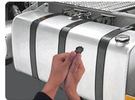
3. Apply force to the patch and squeeze as much as possible into the holes and cracks
