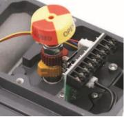
By improving the electrical cam structure, we integrated the four cams into two and separated them with disc springs. The top was compressed with locknuts, which improved the inaccurate positioning of M3 screws by other manufacturers and the difficulty of finding M3 wrenches on the sliding wire site. Disadvantages and can always maintain the stability of the limit in the ultra-high and low temperature environment
