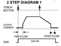
1. Press and hold the Arc Start Switch to start the sequence.
