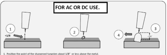
2. Press the torch trigger or press the foot pedal to initiate the arc. The HF arc will be initiated. It may appear briefly as a blue spark.
