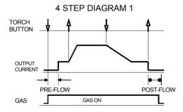
Possible variations of this standard sequence are shown below. By releasing and re-pressing the TIG torch trigger during the downslope step, the output will immediately drop to and hold at the Finish Current. Releasing the trigger will turn off the output and begin postflow. This operation shown in
