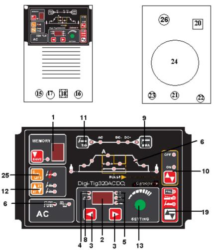
1.Memory chanel LED 2. Data Display meter 3. Parameter Select function 4.indicating light of power 5. S -- unit of up & downslope time & pre& post flow time % -- unit of AC balance &peak time on Hz-- unit of pulse freq.&AC freq.
