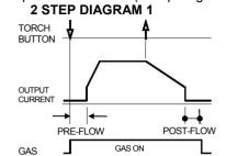
1. Press and hold the Arc Start Switch to start the sequence.
