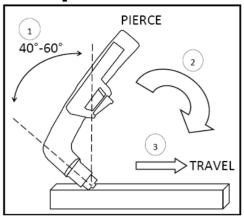
Piercing starts often result in rapid consumable wear and excess blow back of molten metal deposited onto torch and consumables. This should be performed only as necessary.
