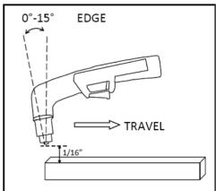
Edge Starts are the best type of start to use if possible to promote consumable and torch life. This reduces blow back of molten material and allows a smooth gradual start of the cut.
