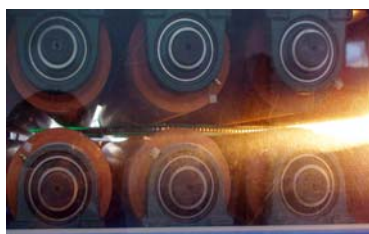
Heat and compaction two glass
