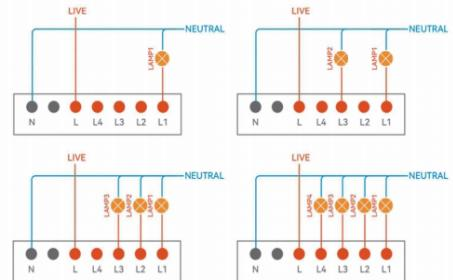
Switch supports single live wire working can be wired in the following way
