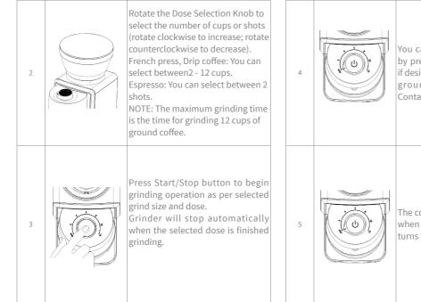
You can pause the Coffee Grinder by pressing the Start/Stop button, if desired. This helps to settle coffee grounds in the Ground Coffee Container.
