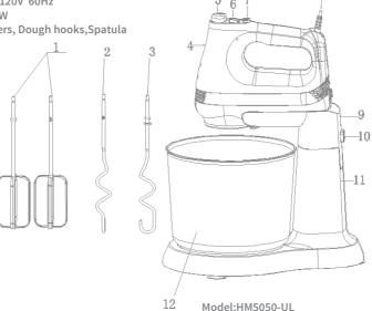
12 Steel Bowl 11 Lower base 10 Release button 9 Bracket 8 Power cord 7 Turbo button 6 Speed selector 5 Ejector button 4 Left Right body 3 Left dough hook 2 Right dough hook 1 beater
