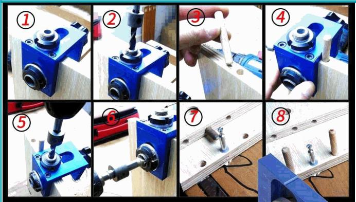
The clamp is adjustable with rotating knob to fit different thickness of wood boards.
