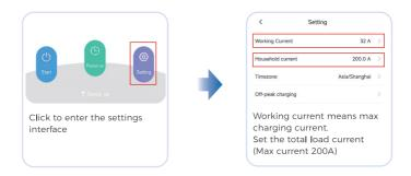
Under this mode, the charger will adjust the real-time charging current according to limitation of 'Househole current', which will avoid the overload.
