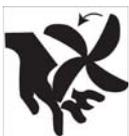
Moving parts, such as fans, rotors, and belts can cut fingers and hands and catch loose clothing.
