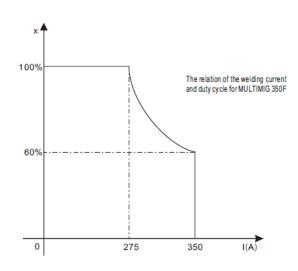
If transformer is over-heat, the heat relay inside it will open and will output an instruction to circuit board, cut AC relay and the output welding current, and brighten the over-heat pilot lamp in the front panel. At this time, the machine should be relaxed for 15 minutes to cool the fan. When operating the machine again, the welding output current or the duty cycle should be reduced.
