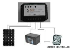
Controller PV+, PV-mouth were connected with the positive and negative PV modules, BAT+, BAT-mouth respectively with positive and negative battery connection, LOAD+, LOAT-DC were loaded with positive and negative connections.
