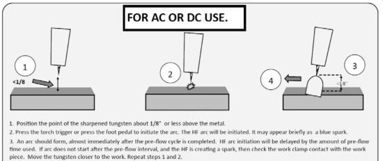
4. Leave 1/8" or less gap between the tungsten tip and the metal and proceed with welding, leaving the torch inclined at a 15° angle.
