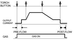
Possible variations of this standard sequence are shown below. By releasing and re-pressing the TIG torch trigger during the downslope step, the output will immediately drop to and hold at the Finish Current. Releasing the trigger will turn off the output and begin postflow. This operation shown in
