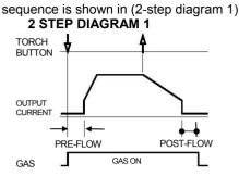
1. Press and hold the Arc Start Switch to start the sequence.
