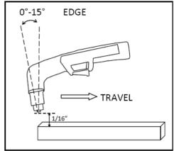
Edge Starts are the best type of start to use if possible to promote consumable and torch life. This reduces blow back of molten material and allows a smooth gradual start of the cut.
