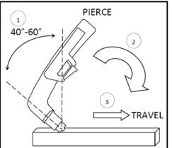
Piercing starts often result in rapid consumable wear and excess blow back of molten metal deposited onto torch and consumables. This should be performed only as necessary.
