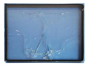
(操作不当,导致中空玻璃炸裂) (Improper operation, resulting in the explosion of the insulating glass) 7. 通常情况下,春夏秋三季热压机加热温度大约在 160 °C -170 °C。冬季热压机加 热温度大约在 200 °C。但实际加热温度要以中空玻璃出热压机后胶条表面温度为 准,该温度为 43 °C -50 °C。如低于该温度,请调高加热温度。如高于该温度,请 调低加热温度。 Under normal circumstances, spring, summer and autumn hot press heating temperature is about 160 °C -170 °C. The heating temperature of hot press
