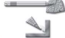
Wrong Tungsten Preparation-Stable Arc
