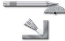
Ideal Tungsten Preparation-Stable Arc
