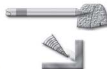
Wrong Tungsten Preparation-Stable Arc
