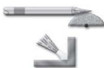
Ideal Tungsten Preparation-Stable Arc
