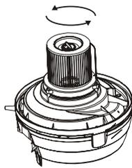
Twist the locking knob with a anti-clockwise force, take off the filters
