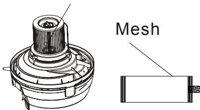
Tear off the mesh outside the HEPA filter
