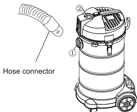
Put the hose connector into ①, the suction function is available
