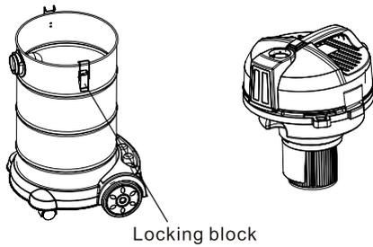
Release the lock block to open the up housing
