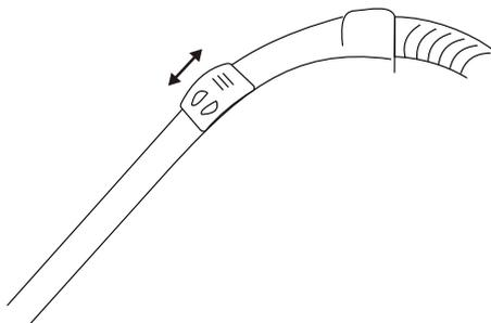
You can adjust the airflow by push the sliding block up and down.
