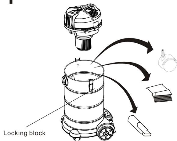
Release the lock block to open the up housing, take out wheels and accessories.
