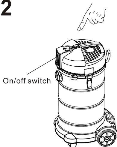
Press the switch button to turn on/off the cleaner
