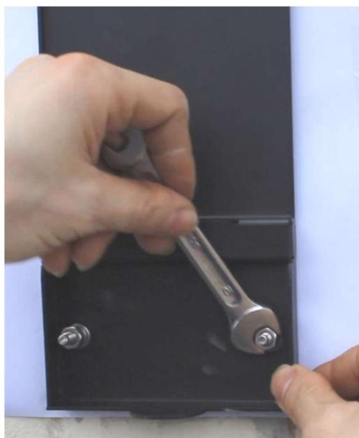
5. Tighten the top screws with a wrench.
